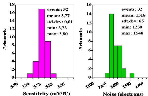
Figure 2: Sensitivity and noise of bare ASIC.
