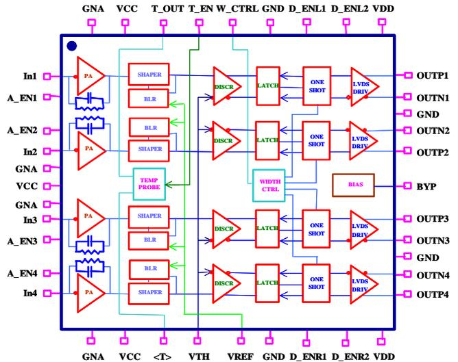
Figure 1: Block diagram of the ASIC.
