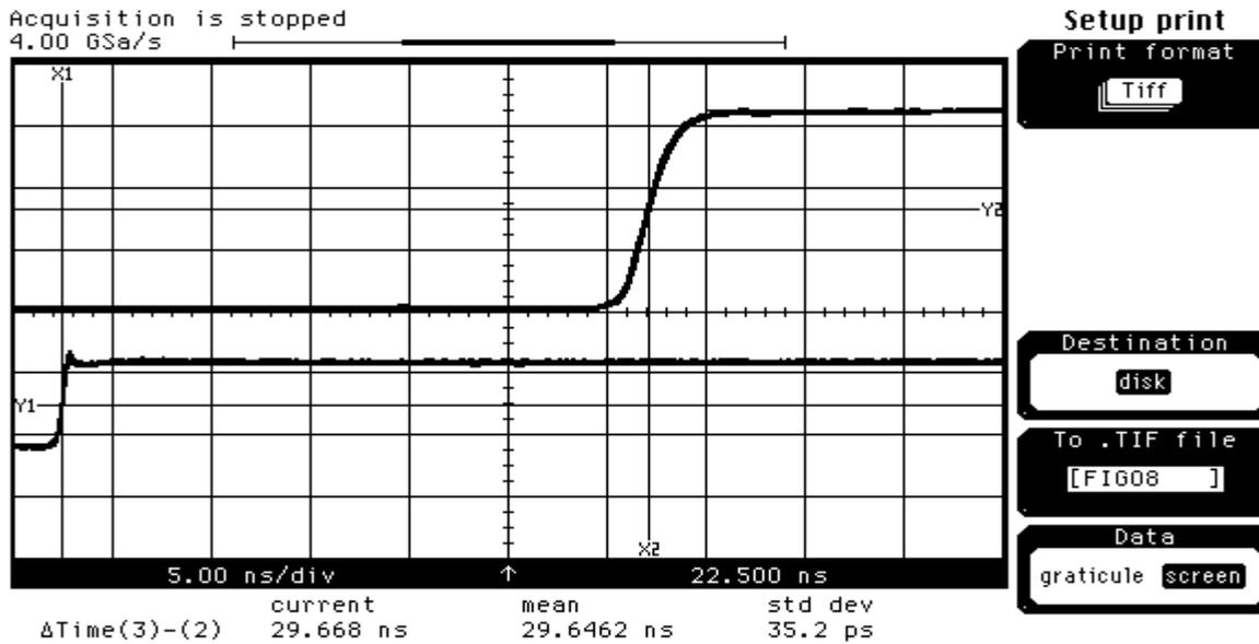
From these pictures one can see that most of the time walk occur for input signals ranging from 1 to 10 fC where the delay between the trigger of the pulse generator and the output from the MAD changes of 3.6 ns.
