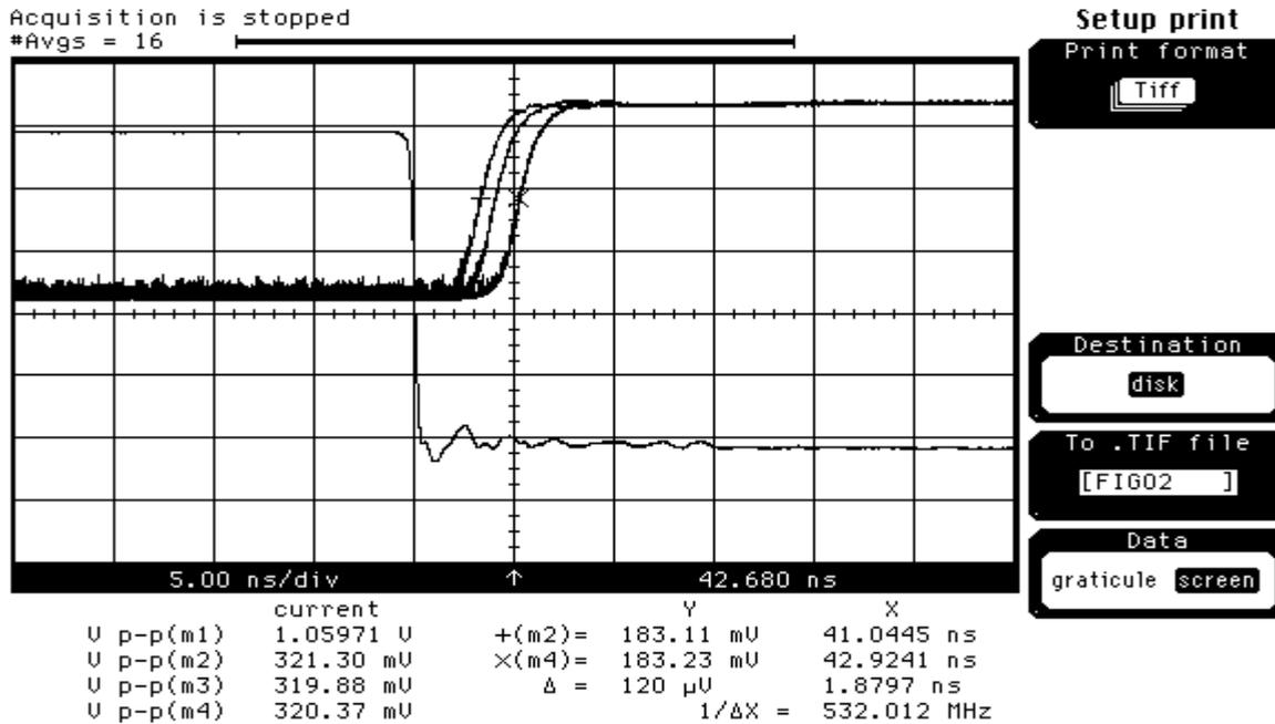
The following pictures show the intrinsic time resolution limited by the preamplifier and discriminator noise evaluated for 1 chip; also in this case the effective input charge is considered while threshold has been set at the lowest attainable value (0.5 fC) for all measures.
